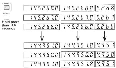
The frequency scans to the lower edge and returns to the higher edge in the desired steps until you push the key.
