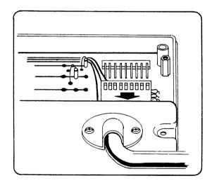
3. Remove the 7th contact pin of P2 from it's molded plastic housing.
